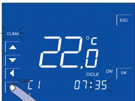
Tap the ▶ key and set the switch-on hour and minute.
