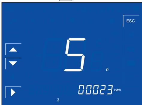
The energy consumption in Kw will be displayed as well as the heating and the connection time of the heating/cooling accumulated for the current day
