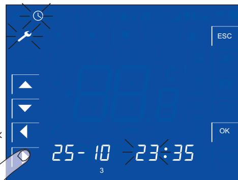
Use the keys to scroll through the different fields (day, month, hour and minutes) and use the keys to adjust the value of the parameters to be modified.
