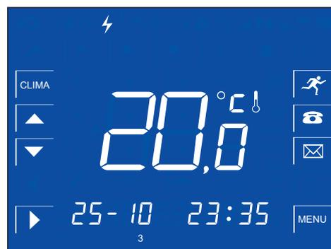
Home screen with the power failure alarm activated.
