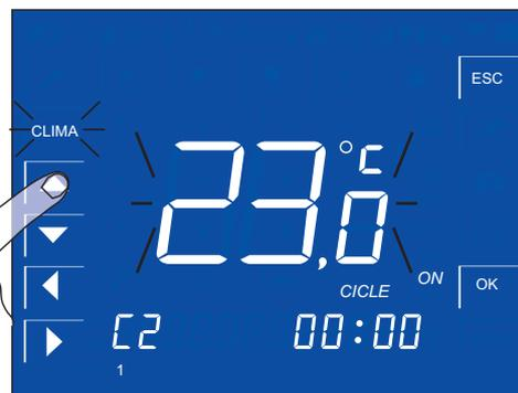
Use the ▲ key to increase the temperature set-point of the next cycle C2 by one degree .
