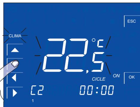
Use the ▼ key to to decrease the temperature set-point of the next cycle C2 by half-a-degree.
