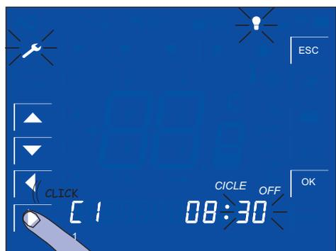
Tap the key and set the lighting switch-on hour and minute.
