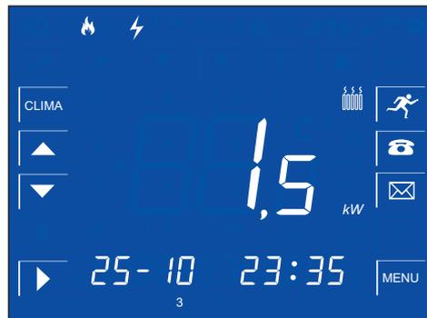
The energy consumption is lower than the threshold selected.
