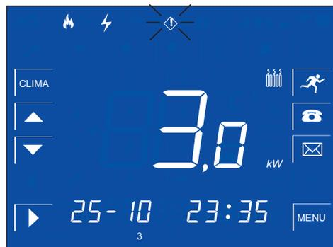
The energy consumption is higher than the threshold selected. The excess of consumption symbol, will be blinking
