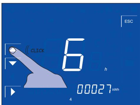
Use the **▲** **▼** keys up to view the connection time of the heating/cooling as well as the energy consumption for the last 7 days.
