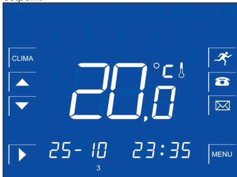
After 5 seconds without changing the temperature set-point the system will automatically display the room temperature.
