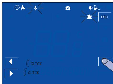
Use the **◀ ▶** keys up to be positioned in the ⚡ icon and the tap the **OK** key.
