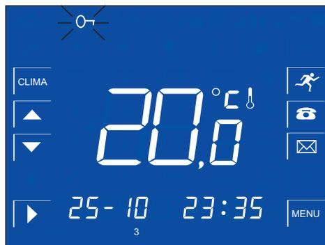
While the alarm is switching on, the icon will be blinking and you will hear a beep sound.
